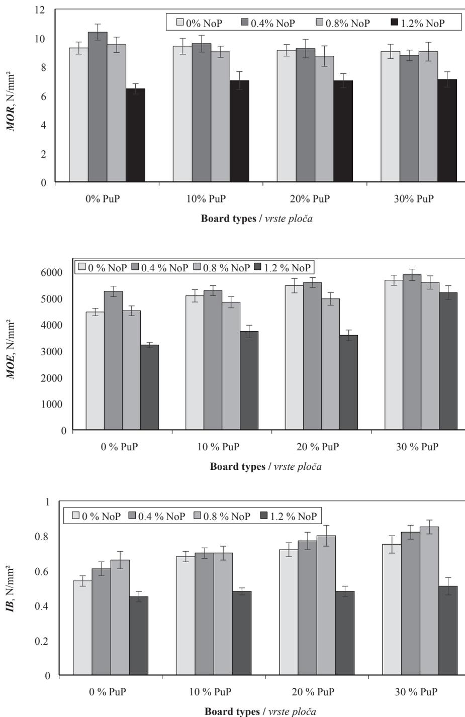
**Figure 2** The effect of the amount of PuP and NoP on mechanical properties of boards
