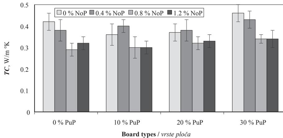
**Figure 3** The effect of the amount of PuP and NoP on thermal conductivity of boards
