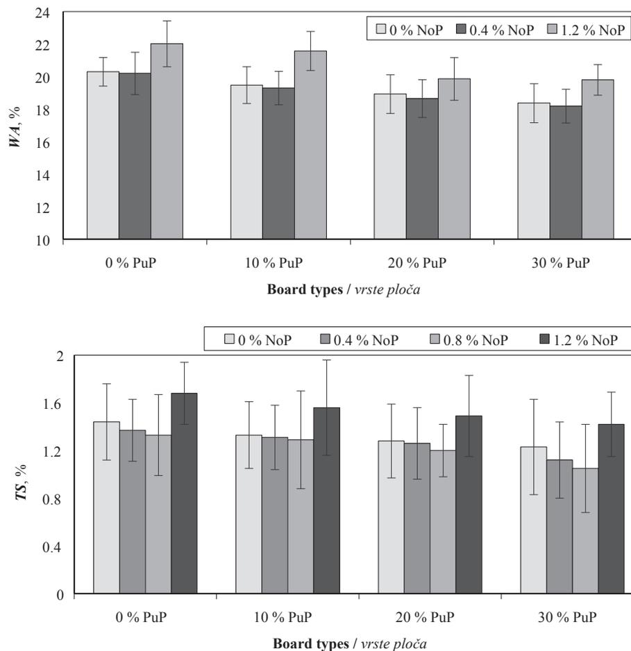
**Figure 1** The effect of the amount of PuP and NoP on dimensional stability of boards
