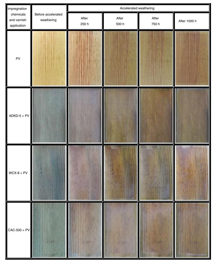
Colour changes of impregnated and polyurethane varnish (PV)-coated Scots pine samples before and after each accelerated weathering period. AD-KD-5, Adolit KD 5; CAC, Celcure AC-500; CV, cellulosic varnish; PV, polyurethane varnish; WCX, Wolmanit CX
