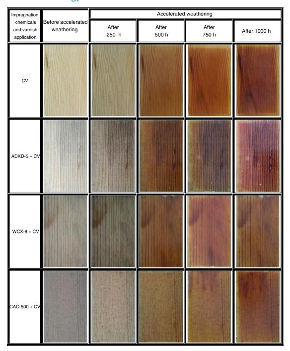
FIGURE 2 Colour changes of impregnated and cellulosic varnish (CV)-coated Scots pine samples before and after each accelerated weathering period. AD-KD-5, Adolit KD 5; CAC, Celcure AC-500; CV, cellulosic varnish; PV, polyurethane varnish; WCX, Wolmanit CX
