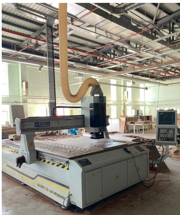
Fig. 1 The 4-axis CNC router, model 2128, manufactured by Megatron
