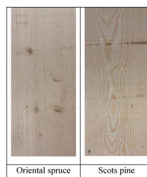
Fig. 3 Oriental spruce and Scots pine cross-sectional images
