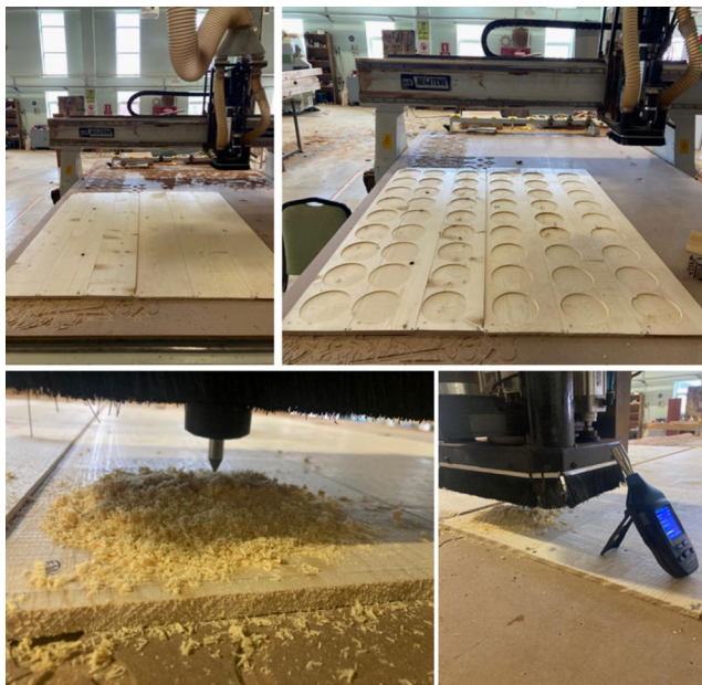
Fig. 7 Wood samples treated with CNC machine and particle measurement device
