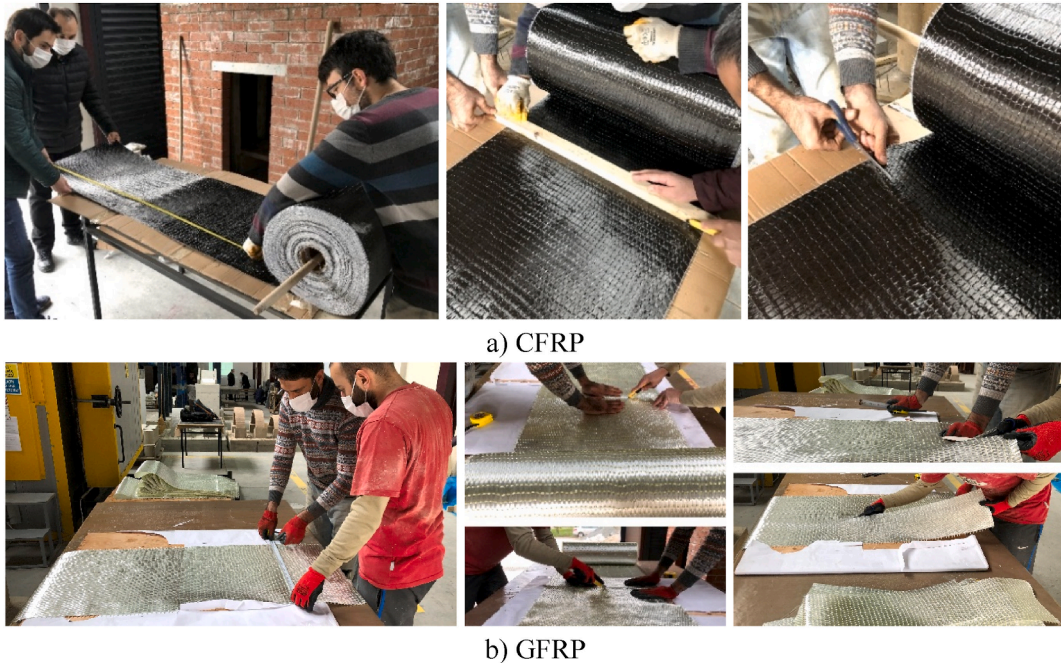
Fig. 2. Preparation of FRP
