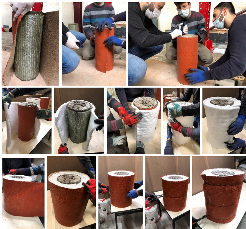
Fig. 7. Wrapping applications of the insulation layers.
