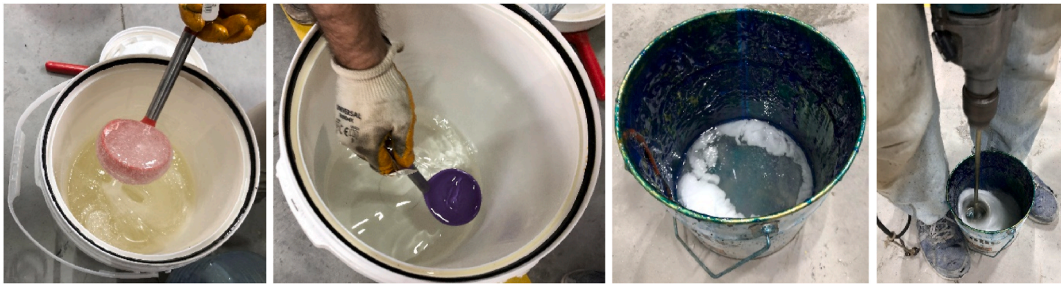
Fig. 3. Preparation of epoxy matrix (epoxy resin and its hardener).
