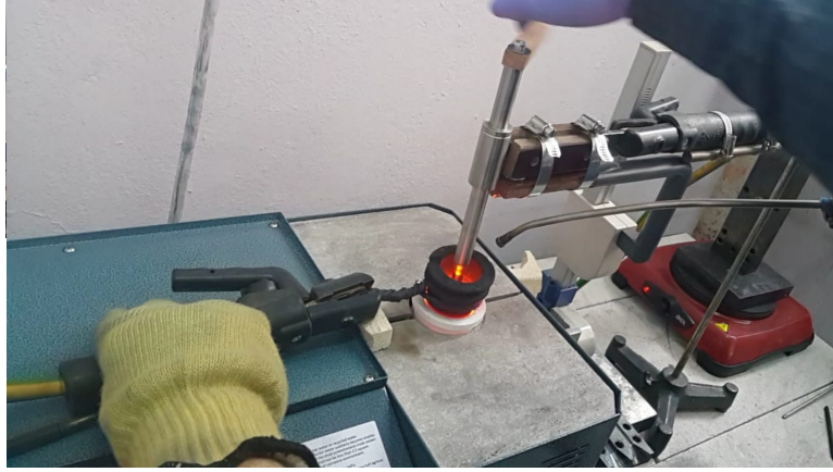
Figure 7: The experimental preparation of the Cu-covetic material.
