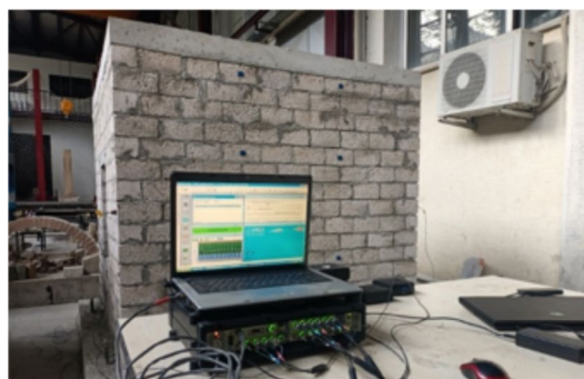
Fig. 7 The setup and location of the accelerometers for the ambient vibration test
