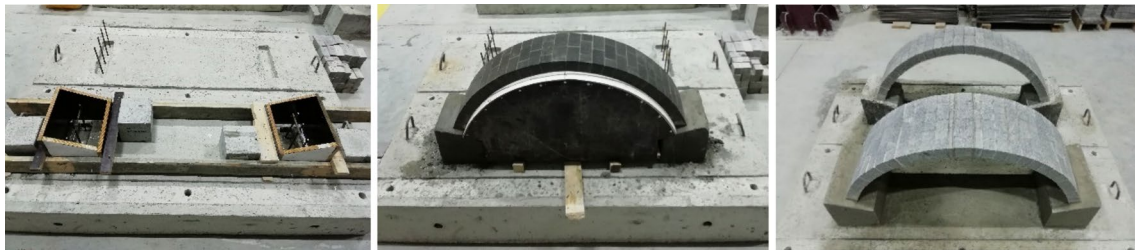
Fig. 3 Construction stages of the arch models
