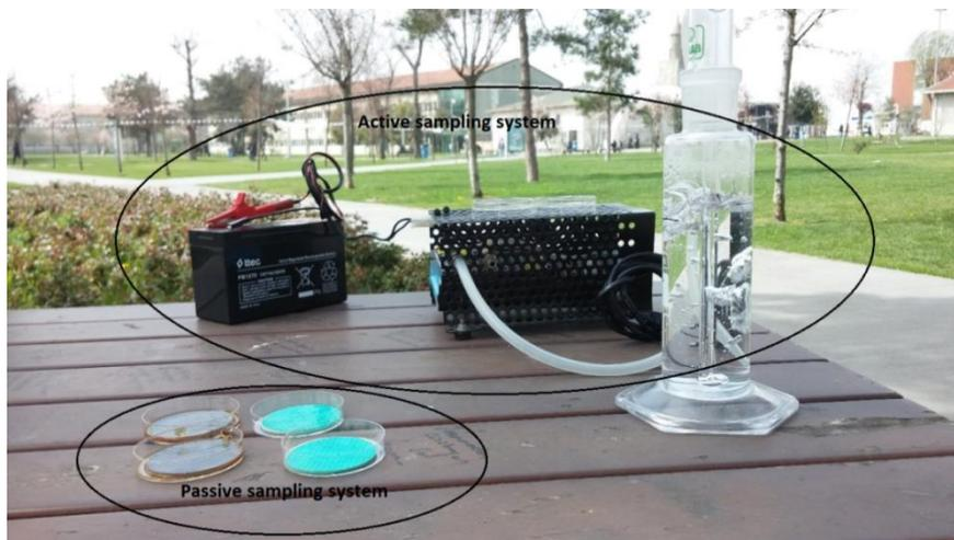
**Figure 1.** Active and passive sampling systems.
